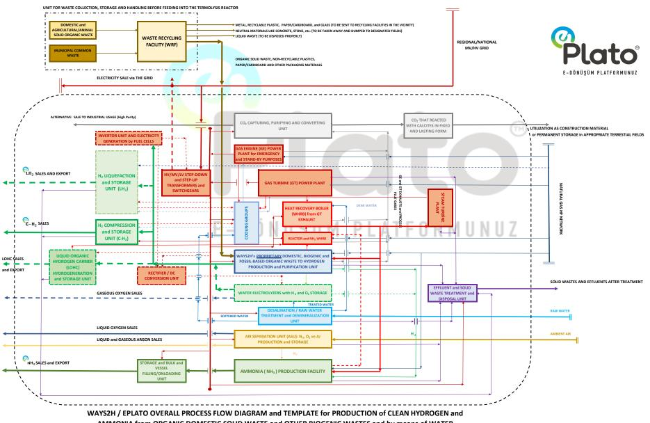
VAYS2H / EPLATO OVERALL PROCESS FLOW DIAGRAM and TEMPLATE for PRODUCTION of CLEAN HYDROGEN and AMMONIA from ORGANIC DOMESTIC SOLID WASTE and OTHER BIOGENIC WASTES and by means of WATER ELECTROLYSIS with RENEWABLE ELECTRICITY
